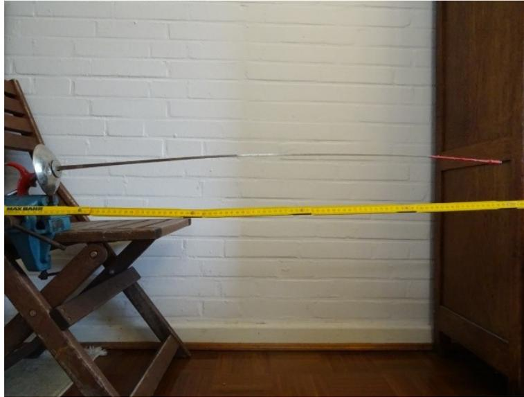
Fig. 2. Mounting of test objects before measurement (shown via the example for the fleuret)
