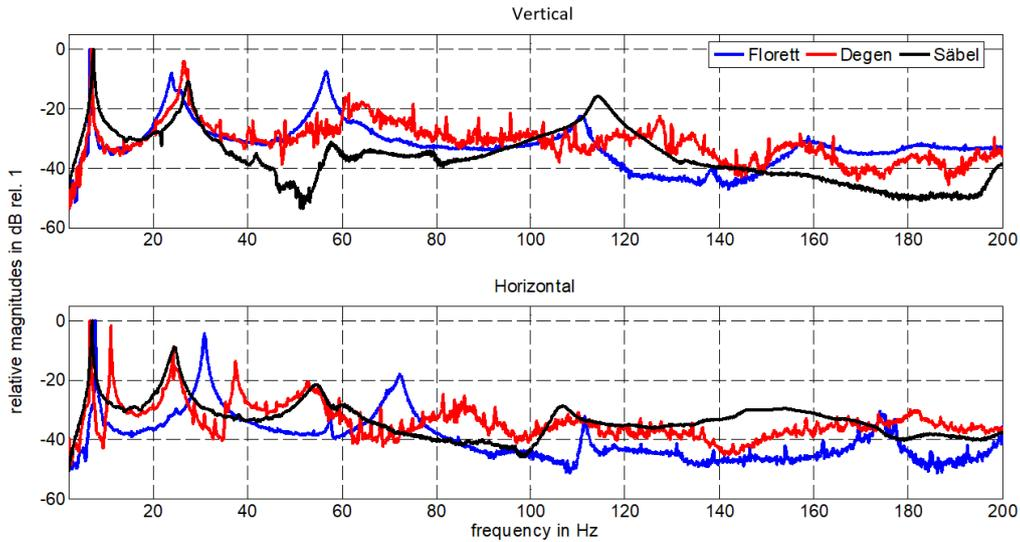
Fig. 6. Frequency response for fleuret (blue curve), épée (red curve) and sabre (black curve) in the lower frequency range
