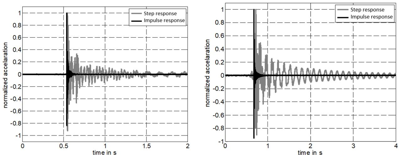
Fig. 3. Free vibration of *épée* (left) and *sabre* (right). Impulse response (black line), Step response (gray line)
