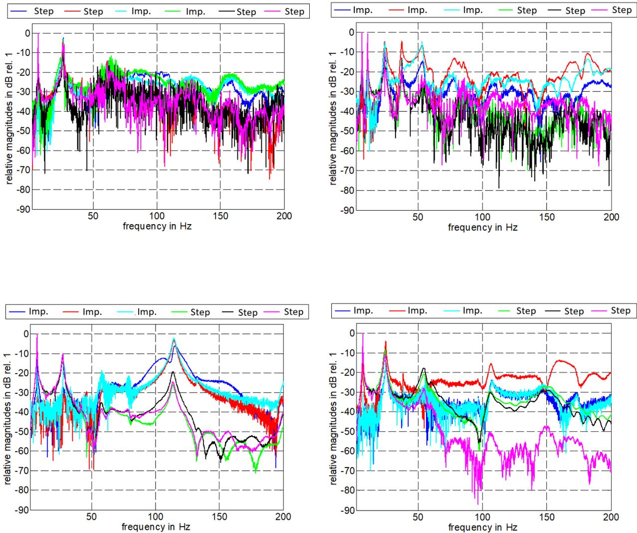
Fig. 5. Magnitude response calculated for impulse input (Imp.) and step input (Step) for fleuret (top), épée (middle) and sabre (bottom). Left column – vibration in vertical direction, right column – vibration in horizontal direction
